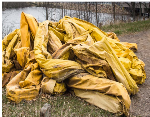
Figure 4. Drying techniques must not trap water. This equipment will not dry adequately. Photo credit: Peter Leete, DNR
